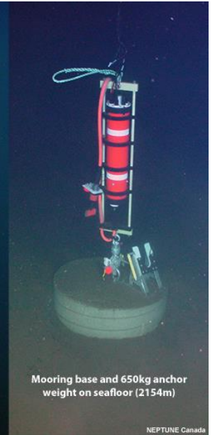
Co-located CTDs and ACMs: 1954, 2029, 2104 & 2149m below sea level; 200, 125, 50 & 5m above the seafloor
